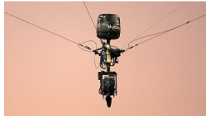
Figure 1.1.5: The gravitational forces and the tension forces on the skycam all act through a single point, making this a concurrent force system that can be analyzed as a particle. Image by Despeaux CC-BY-SA 3.0.
