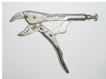
Figure 5.1.4: Many pieces within this pair of locking pliers have forces applied to them at more than two locations. The pieces can also move relative to one another, so this is an example of a machine. Image by Duk CC-BY-SA 3.0
