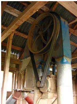
Figure 6.7.1: In many belt-driven systems, the belt friction keeps the pulley from slipping relative to the belt. This allows us to use belts to transfer forces from one pulley to another pulley. Image by Kiilahihnakone, CC-BY-SA 3.0.
