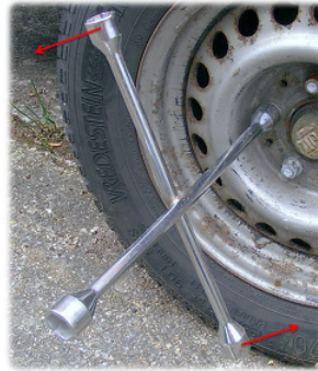
Figure 3.3.1: The two equal and opposite forces exerted on this lug wrench are a couple. They exert a moment on the lug nut on this wheel without exerting any net force on the wheel. Adapted from image by Steffen Heinz Caronna CC-BY-SA 3.0.
