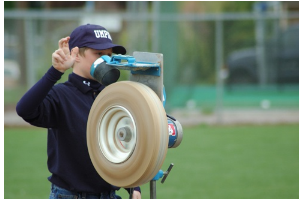
Figure 12.2.1: The wheel on this pitching machine is an example of fixed axis rotation with the axis of rotation at the center of mass. Image by Abigor, license CC-BY 2.0.
