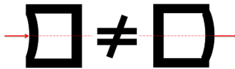
Figure 2.3.2: The exact point of application of a force will impact how internal forces (stresses) are distributed, so the principle of transmissibility cannot be applied when examining internal forces.
