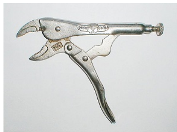
Figure 5.6.4: This pair of locking pliers contains non-two-force members and has parts that can move relative to one another (it is not rigid). Therefore it is a machine. Image by Duk CC-BY-SA 3.0.
