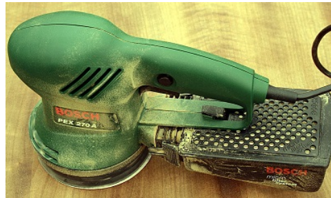
Figure 6.6.1: This orbital sander rotates a circular sanding disc against a stationary surface. The disc friction between the sanding disc and the surface will exert a moment on both the surface and the sander. Image by Hedwig Storch CC-BY-SA 3.0.
