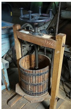
Figure 6.4.1: The screw in this cider press is rotated with the handle on the top. The stationary nut on the frame of the press forces the shaft downward as it is turned. Public Domain image by Daderot.
