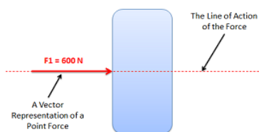
Figure 2.2.5: The line of action of a point force is the line along which the force acts.
