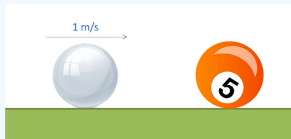
Figure 10.3.2: problem diagram for Example 10.3.1. A cue ball traveling at 1 m/s directly impacts a stationary billiard ball.
