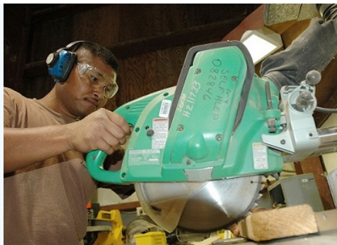
Figure 14.1.3: A man cuts wood with a miter saw. Public domain image by John F. Looney
