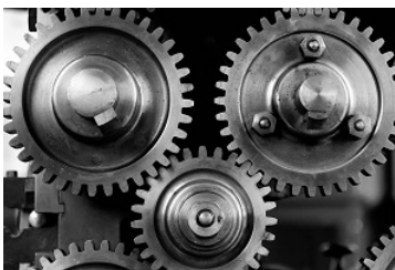
Figure 11.2.2: Gears are another common way of transmitting motion and torque from one shaft to another shaft.
