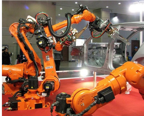
Figure 12.4.1: These robotic arms are a good example of a multi-body kinetics problem. As one section of the arm accelerates, it will exert forces on the other arm sections it is connected to. Image by Chris Chesher, CC-BY-NC-SA 2.0.
