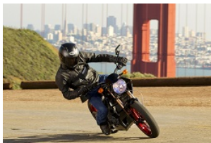
Figure 6.1.2: Dry friction occurs between the tires and the road for this motorcycle. The dry friction force for this motorcycle is what allows it to accelerate, decelerate, and turn. Public Domain image by Takisha Rappold.
