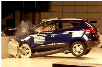
Figure 1.1.2: This car deformed significantly during the crash test. When analyzing the impact, we should not treat the car as a rigid body. Image by Brady Holt CC-BY-3.0.
