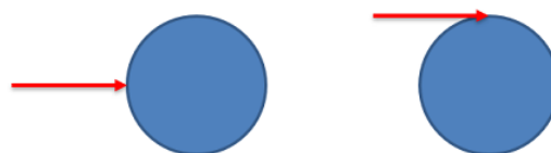
Figure 14.1.1: If we have two identical spheres with forces as shown above, the force on the left would cause only a linear impulse over time, while the force on the right would cause both a linear impulse and an angular impulse over time.
