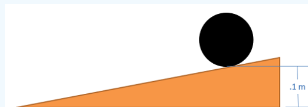
Figure 13.1.5: problem diagram for Example 13.1.3. A spherical ball is placed at the top of a ramp, 0.1 meters above the ground, and rolls without slipping.
