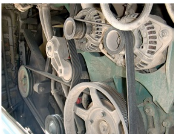
Figure 11.2.1: Belts and pulleys are often used to transmit motion and torque from one shaft to another.
