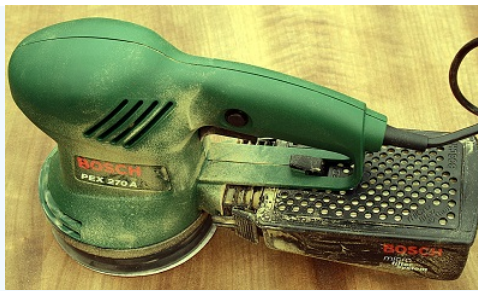
Figure 6.6.6: problem diagram for Example 6.6.1. Orbital sander being used to sand wood. Image by Hedwig Storch CC-BY-SA 3.0.
