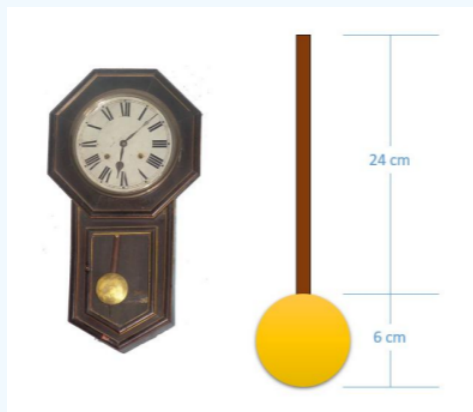
Figure 17.8.10: problem diagram for Exercise 17.8.10. A clock pendulum is represented as a vertical wooden rod with a brass disc attached to its bottom edge.
