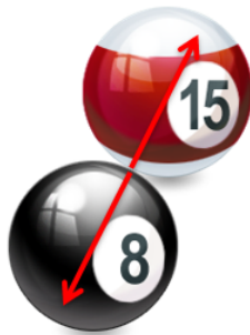
Figure 10.3.1: When two bodies collide, Newton's Third Law ensures that the normal forces from the collision will always be equal and opposite. This means that the impulses will be equal and opposite and will cancel out in our impulse-momentum equation when examining the system of equations.
