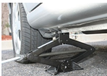
Figure 6.4.2: By rotating the screw in this scissor jack, the user can move the nut (on the left end) closer or further from the anchor on the right end, which will raise or lower the car. Public Domain image by nrjfalcon1.
