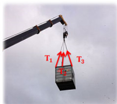
Figure 2.2.1: The tensions in the cables supporting this container can be treated as point forces pulling in the direction of the cables. Adapted from Image by maxronnersjo CC-BY-SA 3.0.
