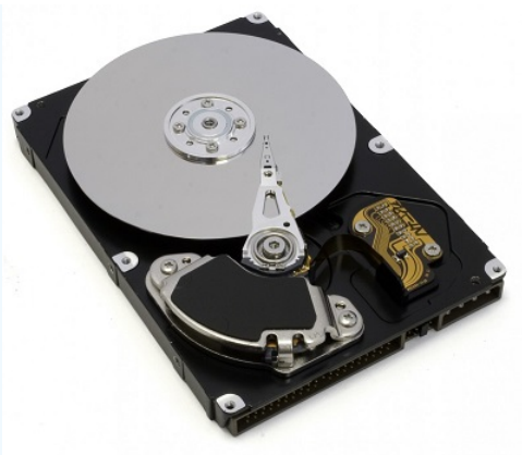
Figure 12.2.3: A picture of a hard drive that emphasizes the flat circular platter.
