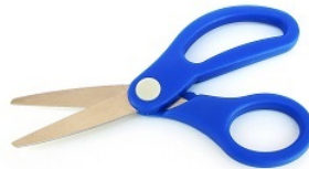
Figure 1.1.3: This pair of scissors consists of two halves held together with a rivet. Because the two halves can move relative to one another, the pair of scissors as whole should not be treated as a rigid body. Image by ZooFari CC-BY-SA 3.0.
