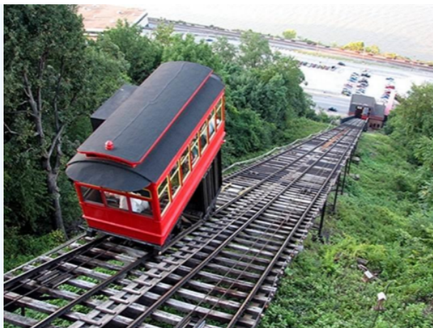
Figure 9.4.3: The Duquesne Incline, a cable car that transports passengers up a steep hillside.
